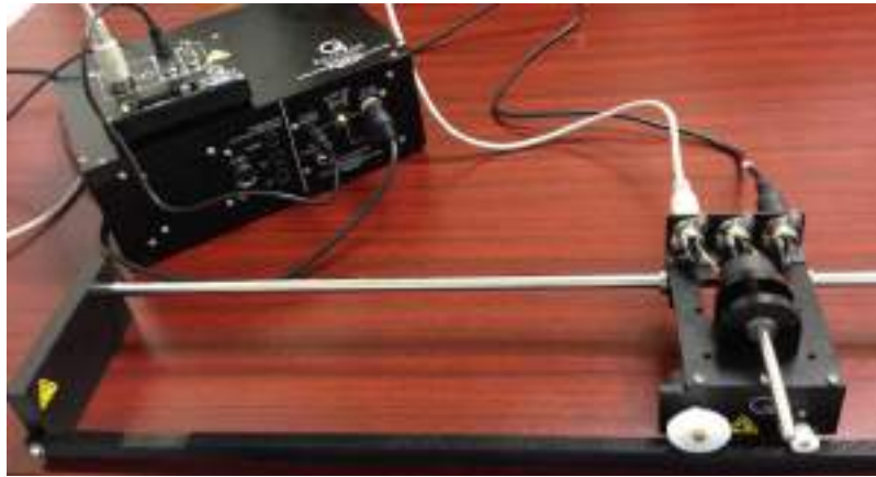
Fig. 10. The IP02 linear motion plant (Manual, 2012).
