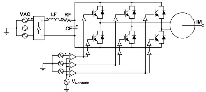
Fig. 5 Circuit schematic.
