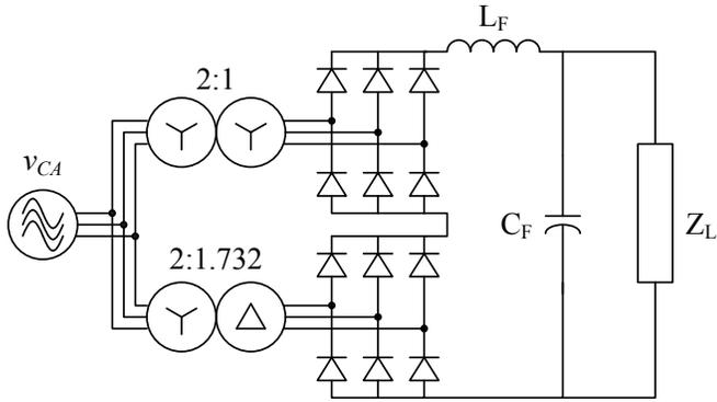
Fig. 6 Adjustable speed drive with a 12-pulse front-end.
