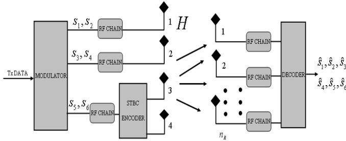
Fig. 1. ZF-QR-OSIC LDSTBC Transmitter/Receiver.
